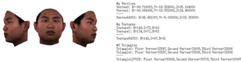
(a) 3D face in different perspectives (b) 3D face data's storage format
